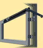
A turning vent pane of a turning door
